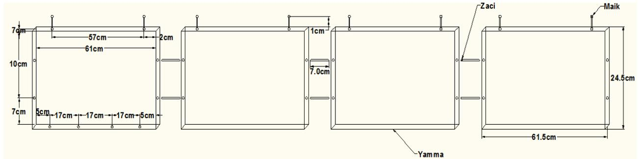
Figure 4. The use of *Zaki* and *Maik* in the construction, and how the four *Yammas* were coupled together
